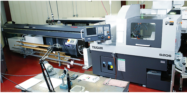
Tsugami S206 6-axis opposed gang tool CNC lathe at Thomas W. Springer
